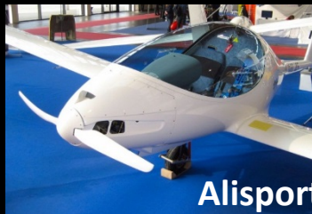
Folding LEAPTech Low Tip Speed Propeller
